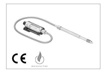
The KE Series are for use in high temperature applications where the process temperatures may reach 538°C (1000°F) such as high temperature engineered polymers. The K Series utilizes standard melt pressure principles and construction, but uses a near incompressible NAK (Sodium Potassium) for pressure transmission. The K Series strain sensing technology is bonded foil strain gage.
