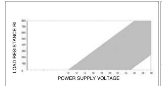
The diagram shows the optimum ratio between load and power supply for transmitters with 4...20mA output. For correct function, use a combination of load resistance and voltage that falls within the shaded area.
