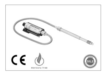
The KE Series are for use in high temperature applications where the process temperatures may reach 538°C (1000°F) such as high temperature engineered polymers. The K Series utilizes standard melt pressure principles and construction, but uses a near incompressible NAK (Sodium Potassium) for pressure transmission.
