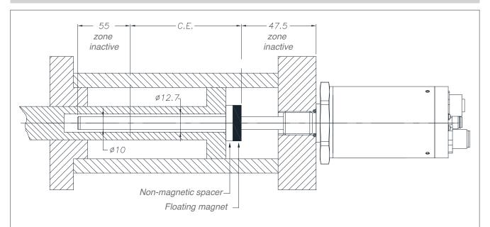
\* for strokes up to and including 1000 mm - over 1000 mm, the inactive zone becomes 60 mm because the tip includes an M4 threaded hole
